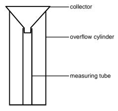
The standard rain gauge shown above has a long, narrow measuring tube and a funnel-shaped collector at the top. The area of the top of the collector is 10 times greater than that of the measuring tube. This difference between the cross-sectional area of the measuring tube and the collector is designed to:
